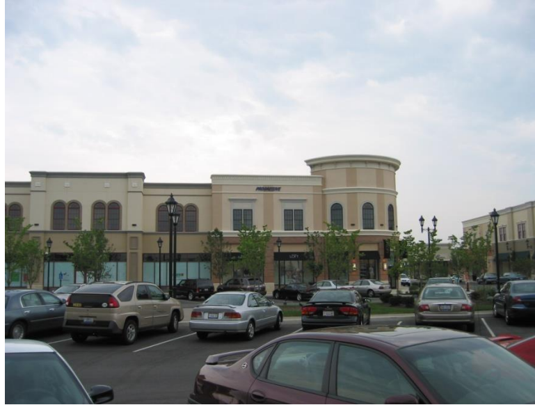
Figure 4: Roofline changes shall be aligned with corresponding wall offsets and/or material or color changes.
